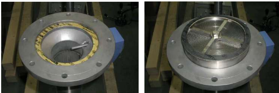
Fig. 8. Installation des joints
